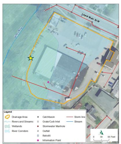
Figure 12. The drainage area for the proposed BMP is shown in orange. The proposed BMP location is shown with a star.
